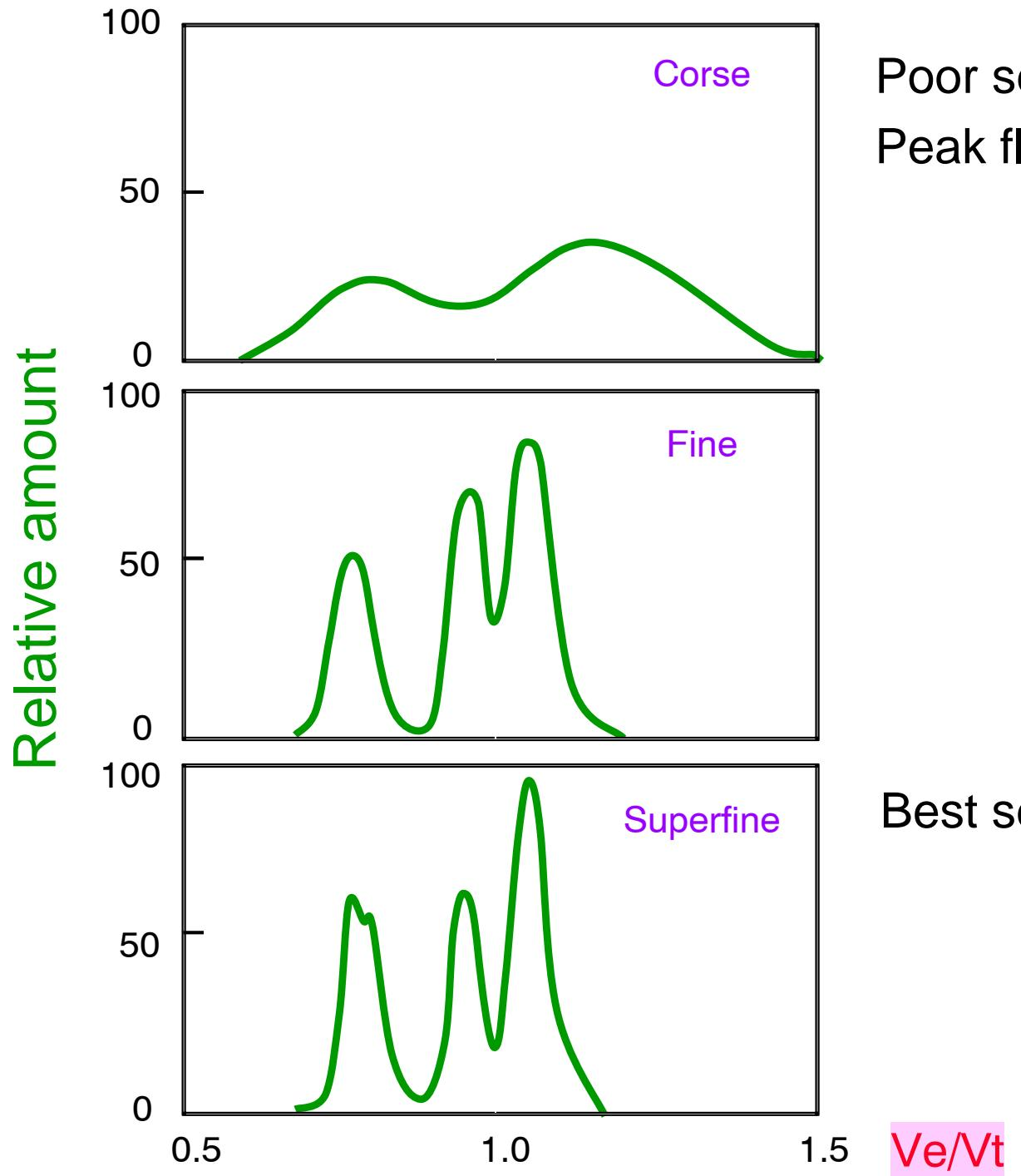
Bead size is critical to the resolution of gel chromatography
