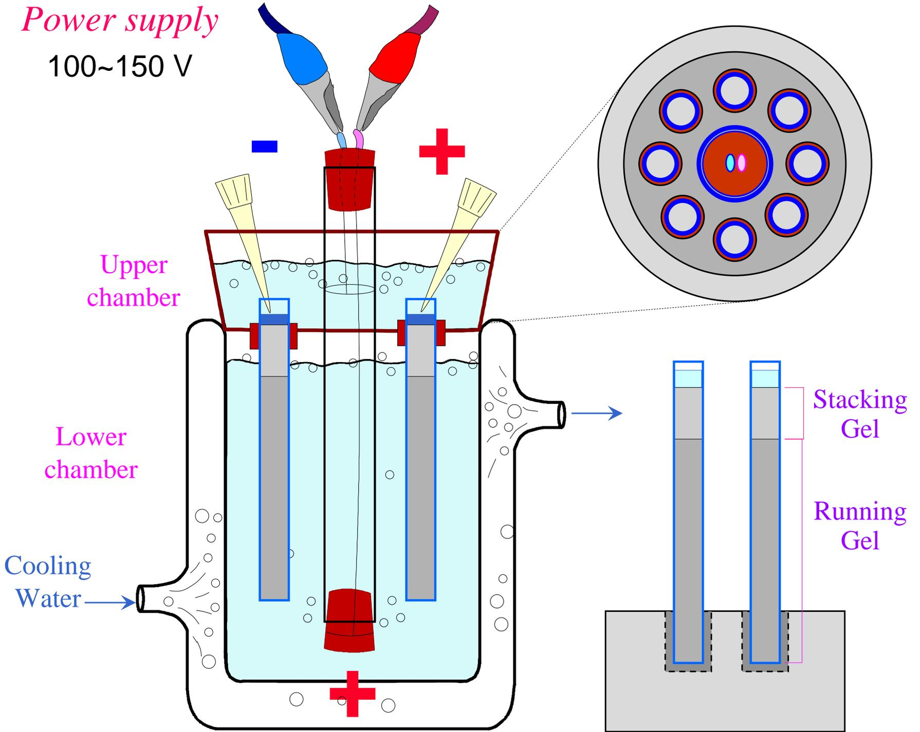
The vertical rod gel is the prototype of modern electrophoresis Juang RH (2005) EPA
