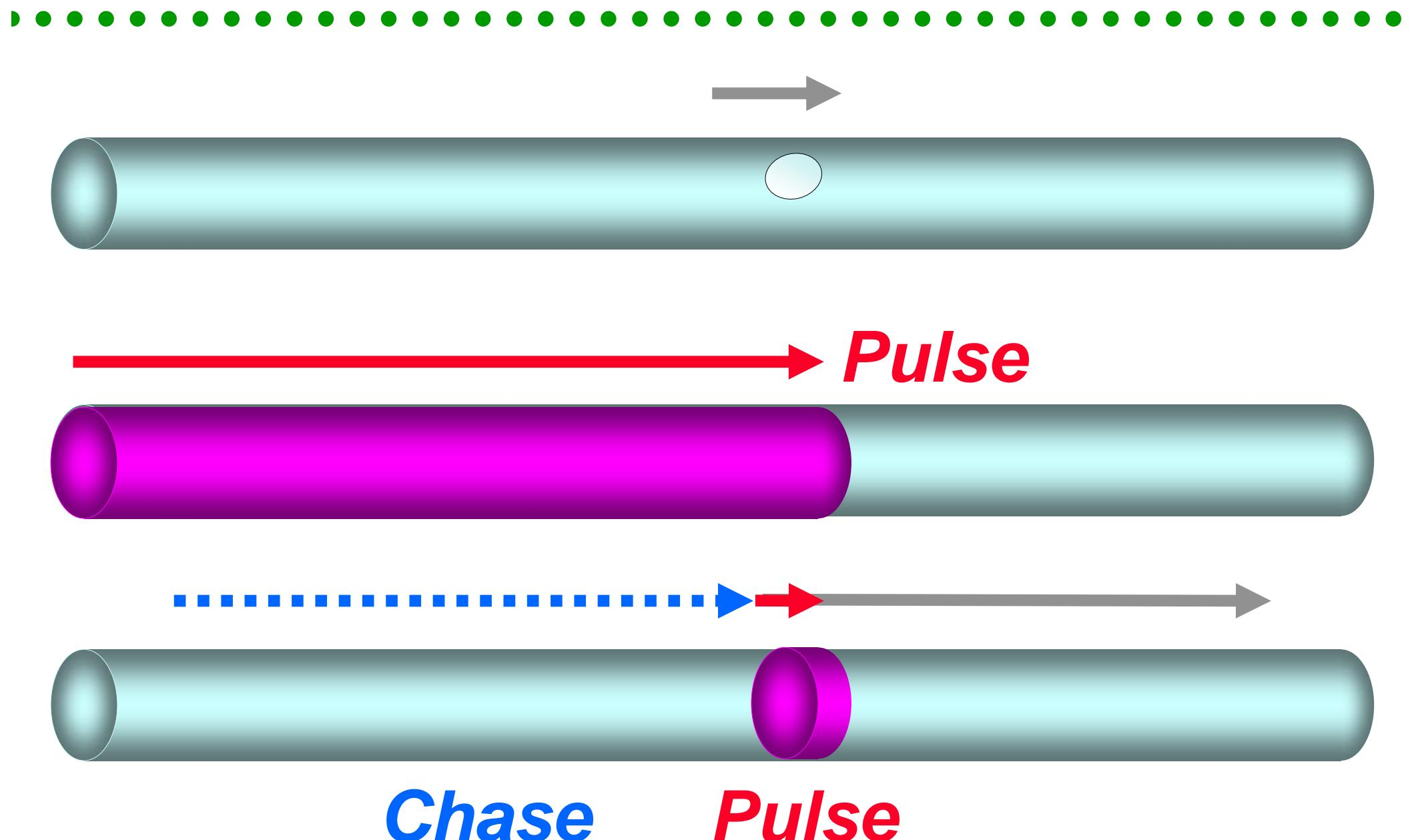
To measure the flow speed of water in a glass tube
