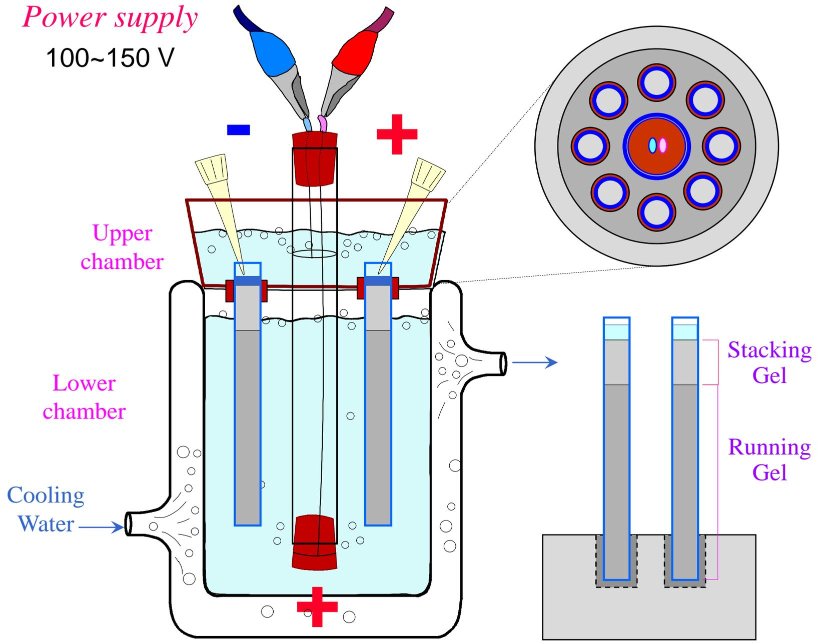
The vertical rod gel is the prototype of modern electrophoresis
